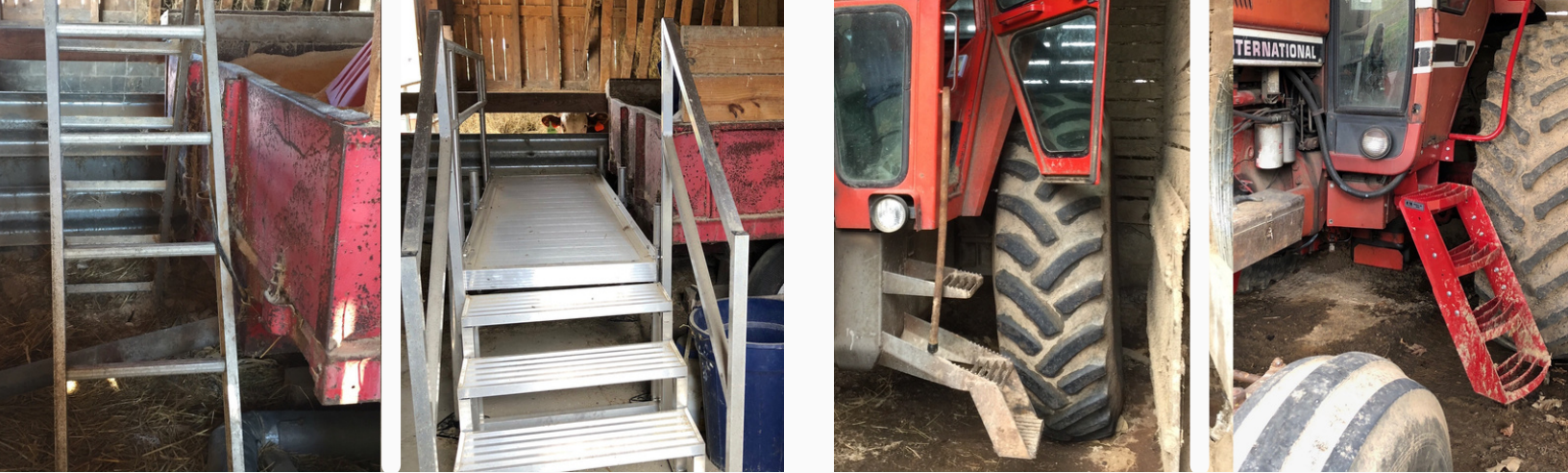
Examples of before and after a worksite assessment. Left Photos: A farmer now uses a stable platform with handrails versus a leaning ladder for accessibility. Right Photos: Additional steps and handrail allow for greater stability when accessing the tractor.
