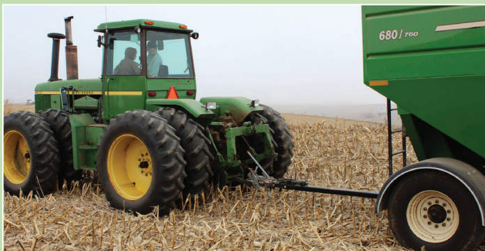
An example of an Agri-Speed Hitch being used with a tractor and wagon, similar to how Bob uses it.
